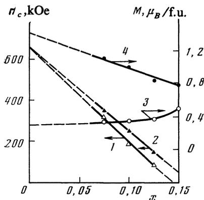
FIG. 5. Concentration dependence of the fields  $H_{c1}$  ( $\Delta$ ) and  $H_{c2}$  ( $\blacktriangle$ ) at which the metamagnetic transition begins and ends, and the magnetic moments at  $H = H_{c1}$  and  $H_{c2}$  ( $\circ$  and  $\bullet$ , respectively);  $T = 4.2$  K.
