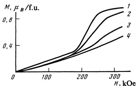
FIG. 4. Magnetization curves for  $\text{Y}(\text{Co}_{0.90}\text{Al}_{0.10})_2$  for  $T = 4.2$  (1), 40 (2), 60 (3), and 80 K (4).
