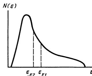
FIG. 1. Rough sketch of the state density curve  $N(\epsilon)$  for  $\text{YCo}_2$ ; the values were calculated by hybridizing the  $4d$  yttrium band with the  $3d$  cobalt band;  $\epsilon_{F1}$  is the Fermi level in  $\text{YCo}_2$ ,  $\epsilon_{F2}$  is the shifted Fermi level after substitution of aluminum for cobalt.
