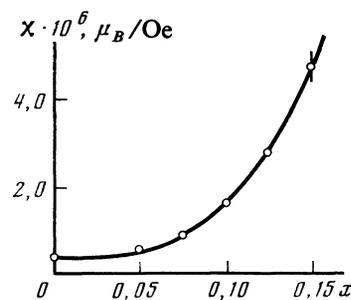
FIG. 3. Paramagnetic susceptibility of  $\text{Y}(\text{Co}_{1-x}\text{Al}_x)_2$  as a function of  $x$ ;  $T = 4.2$  K.
