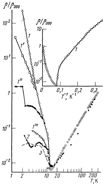
FIG. 2. Temperature dependences of the relative resistivity for different values of direct and microwave currents: 1— $I = 1 \mu\text{A}$ , 1'— $I = 1 \text{ mA}$ , 1''— $I = 10 \text{ mA}$ , 1'''— $I = 30 \text{ mA}$ , 2— $10 \text{ GHz}$ , 3— $9.1 \text{ GHz}$  (results of Ref. 6).
