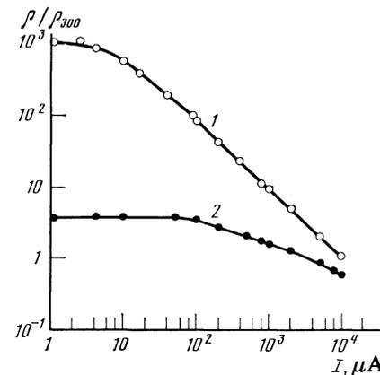
FIG. 3. Current dependence of the relative resistivity: 1— $T = 1.3 \text{ K}$ , 2— $4.2 \text{ K}$ .
