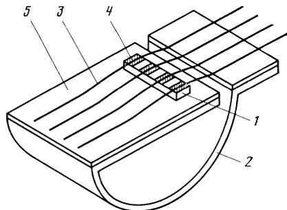
FIG. 1. Mounting and wiring and crystal: 1—crystal, 2—copper foil, 3—platinum-wire electrodes, 4—gold stripes, 5—insulating layer.
