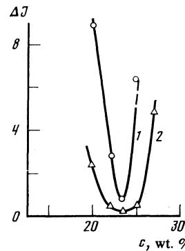
FIG. 3. Temperature-averaged amplitude  $\Delta J$  of the electro-optical polarization of a planar  $C^*$  layer at  $E/E_c \ll 1$  for two ac frequencies,  $f = 40 \text{ Hz}$ ,  $D = 250 \text{ V/cm}$  (curve 1) and  $f = 10 \text{ kHz}$ ,  $E = 1500 \text{ V/cm}$  (curve 2), as a function of the HOBACPC concentration.
