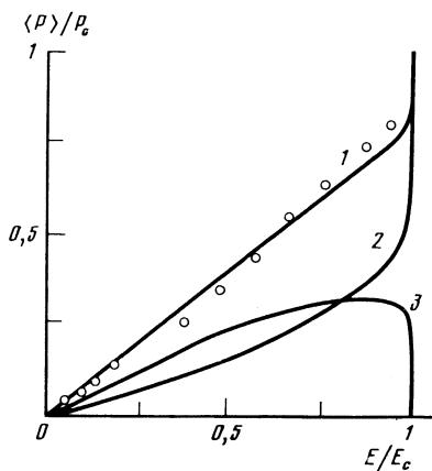
FIG. 4. Least-squares approximation of the experimental  $\langle P \rangle / P_0$  dependence on  $E/E_c$  by the theoretical relation (11) for  $T_c - T = 0.7^\circ\text{C}$  and  $\beta = 0.7 \cdot 10^3$ . O experiment, solid curve 1—calculated data. The relative deviation of the theoretical values from experiment does not exceed 20%. Curves 2 and 3 show the piezoelectric and flexoelectric contributions to the polarizations, respectively, as calculated from Eq. (11).
