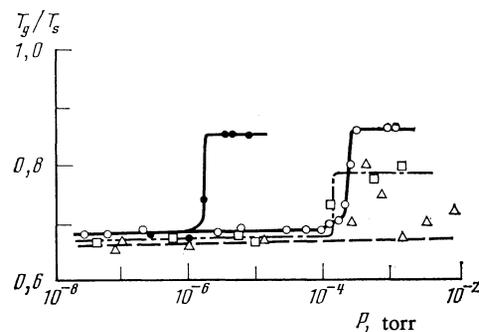
FIG. 3.  $T_g$  versus the residual gas pressure  $P$ . ●, ○—Lead; □—bismuth; △—tin.
