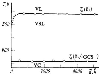
FIG. 8. Diagram of crystal-liquid transitions for Bi constructed from measurements of the resistance. VSL—Vapor-supercooled liquid condensation mechanism.
