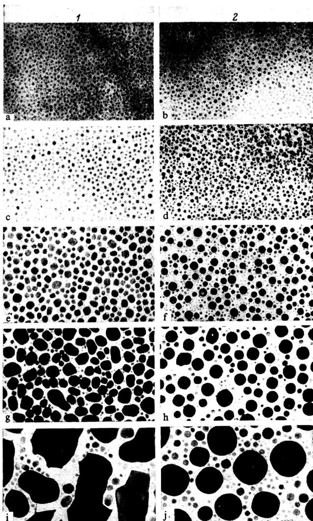
FIG. 2. Electron micrographs ( $10^5 \times$ ) of tin island films on graphite substrates. 1: Vapor-crystal mechanism (320 K). 2: Vapor-liquid mechanism ( $T = 350$  K). The film thicknesses are: a, b—20 Å; c, d—35 Å; e, f—50 Å; g, h—120 Å; i, j—300 Å ( $10^5 \times$ ).
