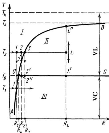
FIG. 6. Diagram of crystal-liquid phase transitions for condensed island films and small particles. VL—Vapor-liquid condensation mechanism; VC—Vapor-crystal condensation mechanism.
