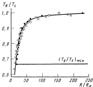
FIG. 9. Generalized diagram of crystal-liquid transitions. O—Au; ●—Pb; □—In; △—Sn.
