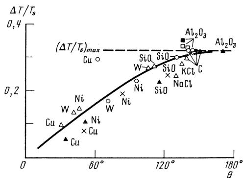
FIG. 5. The relative magnitude of the supercooling versus the wetting edge angle for various metals. The notation is the same as in Fig. 4.
