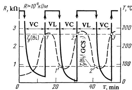
FIG. 7. Electrical resistance (solid line) of Bi films versus the substrate temperature (dashed line) during continuous condensation in a vacuum of  $10^{-8}$  torr. 1, 2, 3—Melting of the films; 1', 2'—crystallization. GCS is a glass ceramic substrate.
