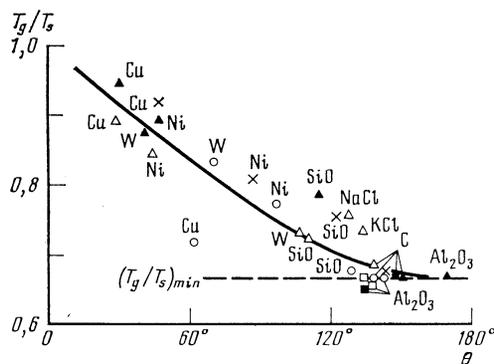
FIG. 4. The relative temperature  $T_g/T_s$  versus the edge angle ( $\theta$ ) for the wetting of the substrates by the condensates for various metals:  $\square$ —Ni,  $\circ$ —Co;  $\blacksquare$ —Fe;  $\triangle$ —Pb;  $\blacktriangle$ —Sn;  $\circ$ —Bi;  $\bullet$ —Au;  $\times$ —In (the points are labeled with the substrate material).
