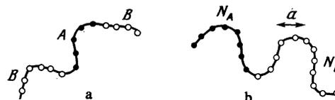
FIG. 1. Triblock copolymer (a) and diblock copolymer (b);  $N_A$  and  $N_B$  are the numbers of links of types  $A$  and  $B$ .
