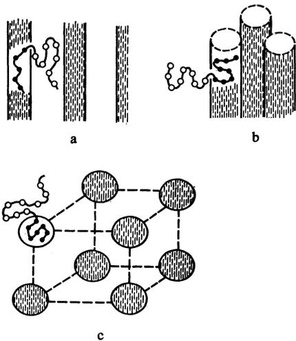
FIG. 2. Microdomain structures: lamellar (a), cylindrical (b), spherical (c).
