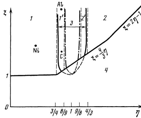
FIG. 3. Values of the parameters  $\eta$ ,  $\xi$  at which the corresponding cross sections are convex or nonconvex—solid lines; boundaries of transition from ordinary to generalized Rayleigh waves—dashed lines (see text). The values of the elastic moduli for nickel, diamond and aluminum were taken from Ref. 1.
