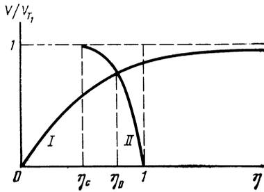
FIG. 1. Dependence of the velocity of Rayleigh waves on the anisotropy parameter (curve I); solution of the equation  $\gamma_1 = \gamma_2$  corresponding to the surface wave (curve II); plane (001), direction of the wave [100].
