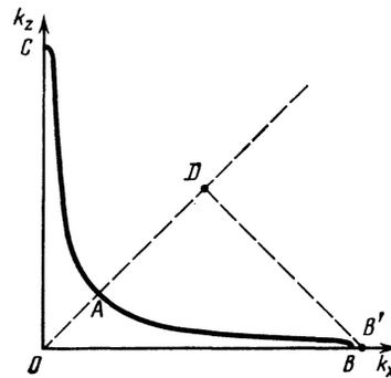
FIG. 5. Cross section in the  $k_x k_z$  plane of the isofrequency surface of the transverse bulk mode  $V_{T_1}$  in the case  $\eta \gg 1$ .
