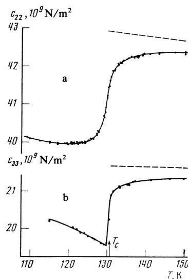
FIG. 2. Temperature dependence of the elastic moduli  $c_{22}$  (a) and  $c_{33}$  (b) in the phase-transition region. Points—experimental values, through which the lines were drawn to emphasize the difference between the behavior of  $c_{22}$  and  $c_{33}$ . Dashed line—expected behavior of  $c_{22}$  and  $c_{33}$  in the paraphase in the absence of fluctuation corrections.
