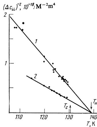
FIG. 4. Temperature dependences of  $(\Delta c_{11})^{-2}$  (curve 1) and of  $(\Delta c_{33})^{-2}$  (curve 2), which characterize the proximity of the phase transition to the tricritical point.  $n = T_n - T_c = 8.5$ .
