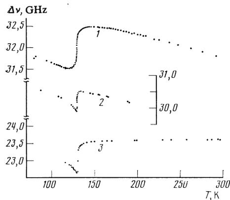
FIG. 1. Temperature dependence of the Brillouin-component shift  $\Delta\nu$ . The light scattering which was investigated was from longitudinal acoustic phonons propagating along the polar axis  $b$  (1),  $c$  (2), or  $a$  (3).
