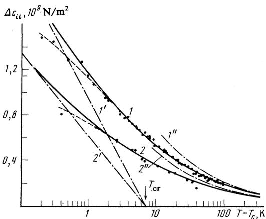
FIG. 5. Semilog plots of the anomalous parts  $\Delta c_{22}$  (1) and  $\Delta c_{33}$  (2) vs temperature in the paraelectric phase. Points—experimental values. The solid curves 1 and 2 were calculated from Eq. (10): 1' and 2'—asymptotes of the form  $\Delta c \propto \ln \tau$ ; 1'' and 2''—asymptotes of the form  $\Delta c \propto \tau^{-5}$ . The dashed lines that meet curves 1 and 2 show that reduced values of  $\Delta c$  are observed at  $T < t - T_C = 2$  K (see the text).
