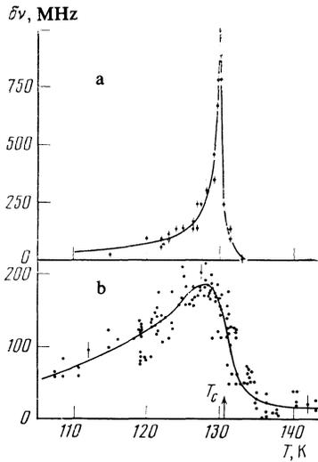
FIG. 3. Temperature dependence of the damping of the longitudinal acoustic phonons propagating perpendicular (a) and parallel (b) to the polar axis. The width  $\delta\nu$  of the Brillouin components measured at half-maximum of the phonon line is shown; the instrumental broadening is subtracted.
