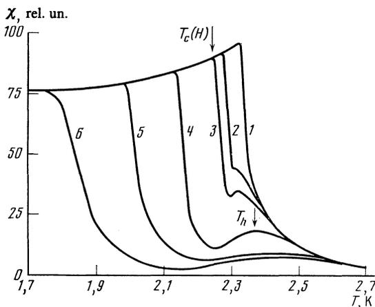
FIG. 1. Temperature dependences of the magnetic susceptibility of  $\text{CuRb}_2\text{Br}_4 \cdot 2\text{H}_2\text{O}$  in the difficult magnetization direction at a pressure 9.5 kbar in dc magnetic fields: 1— $H = 0$ ; 2— $H = 50$  Oe; 3— $H = 70$  Oe; 4— $H = 110$  Oe; 5— $H = 200$  Oe; 6— $H = 250$  Oe.
