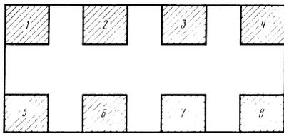
FIG. 2. Sketch showing the arrangement of the contacts used to study the homogeneity of the crystals.
