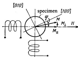
FIG. 1. Mutual orientation of the specimen, search coil, and magnetic field.
