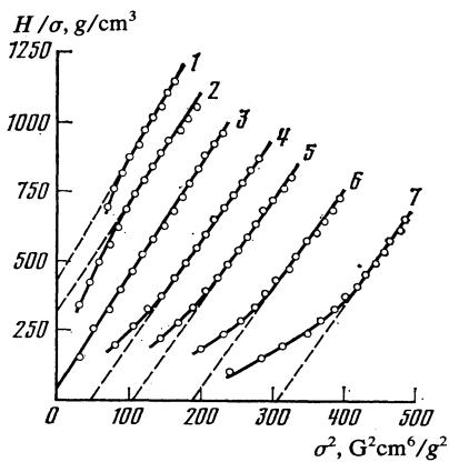
FIG. 4. Dependence of the ratio  $H/\sigma$  on  $\sigma^2$  for  $Mn_{0.4}Cr_{0.6}Sb$  in the vicinity of the canted-ferromagnetic-antiferromagnetic transition. Temperatures in K are: 1) 323; 2) 318; 3) 313; 4) 308.3; 5) 303; 6) 298; and 7) 290.
