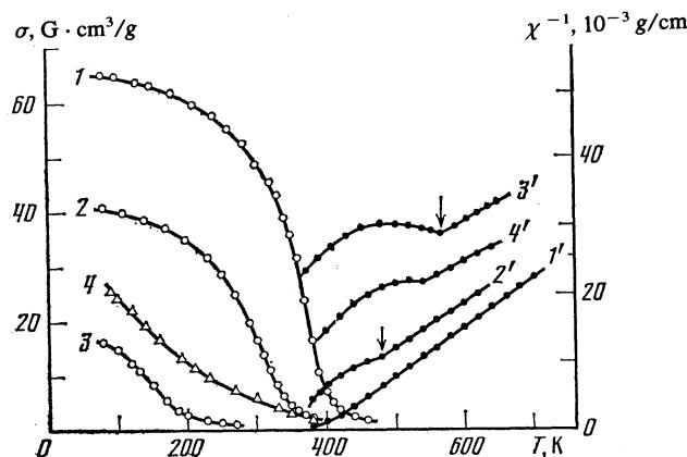
FIG. 5. Temperature dependence of specific magnetization and inverse susceptibility,  $\chi^{-1}$  (curves denoted by primed numbers) for the  $Mn_{1-x}Cr_xSb$  alloys measured in a field of 8 kOe for the annealed alloys: 1 and 1')  $x = 0.5$ ; 2 and 2')  $x = 0.6$ ; 3 and 3')  $x = 0.75$ ; and for the quenched alloy: 4 and 4')  $x = 0.7$ . The arrows indicate  $T_N$ .
