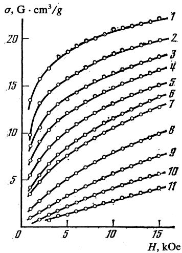
FIG. 3. Magnetization curves of  $Mn_{0.4}Cr_{0.6}Sb$  in the vicinity of the canted-ferromagnetic-antiferromagnetic transition. Temperatures in K are: 1) 290; 2) 298; 3) 303; 4) 308.3; 5) 313; 6) 318; 7) 323; 8) 333; 9) 343; 10) 353; and 11) 368.
