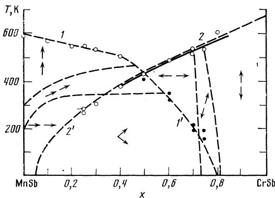
FIG. 2.  $Mn_{1-x}Cr_xSb$  magnetic phase diagram plotted from the temperature dependence of  $\Delta I/I$  (○) and from the magnetic measurements (●). The solid curve corresponds to first-order phase transitions, the dashed curves to second-order phase transitions.<sup>6</sup>
