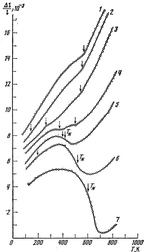
FIG. 1. Temperature dependence of linear thermal expansion of  $Mn_{1-x}Cr_xSb$  alloys. 1)  $x = 0$ ; 2)  $x = 0.1$ ; 3)  $x = 0.25$ ; 4)  $x = 0.4$ ; 5)  $x = 0.5$ ; 6)  $x = 0.7$ ; 7)  $x = 0.8$ . The arrows show  $T_C$  according to the magnetic measurements;  $T_N$  and the temperatures of the canted-structure-ferromagnetic transition (dashed arrows) are determined from neutron diffraction data.<sup>6</sup>
