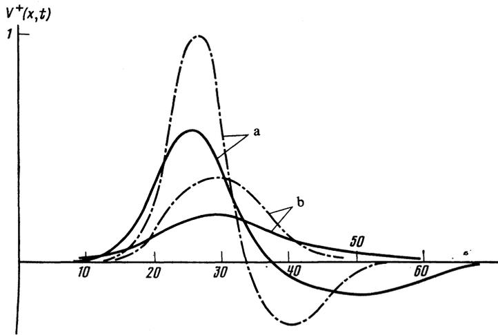
FIG. 1. Rate of SR decay  $V^+(x, t)$  as a function of time: a—near the right edge of the specimen, b—near the center of the specimen  $\tau_R/\tau_0 = 10^{-3}$ ,  $c\tau_R = 3L$ ; dot-dash curves—solution obtained for (18)–(20); solid curves—solution obtained for (15)–(17).
