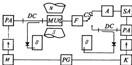
FIG. 2. Block diagram of the experimental setup: *M* is a magnetron oscillator; *PA*, a precision attenuator; *DC*, a directional coupler; *MUG*, the measuring unit with the ferrite; *PG*, a trigger pulse generator; *O*, oscillograph; *F*, filter; *CS*, coaxial switch; *A*, amplifier; *SA*, spectrum analyzer; and *K*, klystron oscillator.
