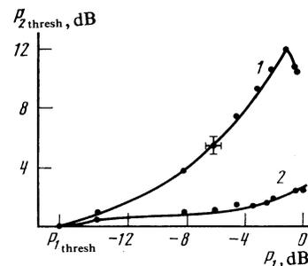
FIG. 3. Dependence of the second pump's threshold  $P_{2th}$  on the first pump's power  $P_1$ : 1)  $\Delta f \lesssim 10$  MHz; 2)  $\Delta f = 15 \pm 5$  MHz (see Fig. 1). 0 dB on the vertical axis corresponds to the quantity  $P_{2th}$  in the absence of the first pump ( $P_1 = 0$ ); 0 dB on the horizontal axis corresponds to the kinetic-instability threshold  $P_{1kin}$  in the absence of the second pump. The sample was a spherical YIG single crystal of 2 mm diam.
