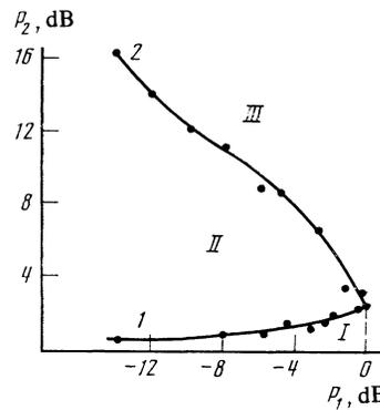
FIG. 5. Stability diagram for the spin waves in the case when  $\Delta f = 15 \pm 5$  MHz. In the region I spin waves with frequency  $\omega_{p1}/2$  are excited; in the region II, spin waves with frequencies  $\omega_{p1}/2$  and  $\omega_{p2}/2$ ; in the region III, spin waves with frequencies  $\omega_{p1}/2$ ,  $\omega_{p2}/2$ , and  $\omega_{k_0} \approx \omega_{\text{min}}$ .
