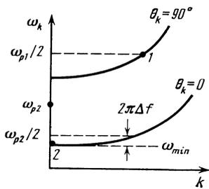
FIG. 1. Disposition of the pump frequencies relative to the spin-wave spectrum: 1) location in the PSW<sub>1</sub> spectrum; 2) location of the spin waves excited as a result of the kinetic instability:  $\omega_{p2}/2$  is the frequency of the PSW<sub>2</sub> and  $\omega_{p2}$  is the frequency of the uniform magnetization oscillation (i.e., of the ferromagnetic resonance) and of the second pump.
