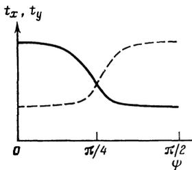
FIG. 1. Characteristic dependence of transmittances  $t_x$ ,  $t_y$  on the slope angle of the radiation polarization (vector on the front face of the crystal relative to the axis of symmetry (see text).
