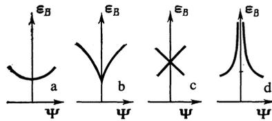
FIG. 2. Angular dependence of the bifurcation value of the amplitude of the field  $\varepsilon$  incident on the cavity at small angles  $\Psi$  between the polarization plane and the axis of symmetry of the crystal: (a) extremum corresponding to absorptive optical bistability; (b) extremum corresponding to dichroic bistability; (c) self-intersection; (d) tendency to infinity.
