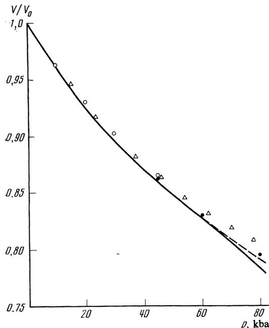
FIG. 3. Pressure dependence of the reduced volume  $V/V_0$  for polycrystalline lanthanum. The solid curve represents the data of the present experiment, the filled circles the data of Ref. 2, the open circles the data of Ref. 6, and the triangles the data of Ref. 7.
