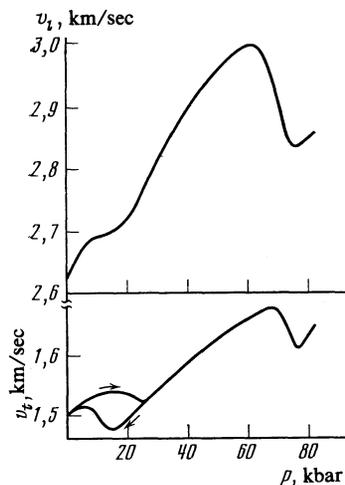
FIG. 1. Pressure dependence of the velocities  $v_l$  and  $v_t$  of longitudinal and transverse ultrasonic waves, respectively, in polycrystalline lanthanum.
