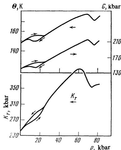
FIG. 2. Pressure dependence of the bulk modulus  $K_T$ , shear modulus  $G$ , and Debye temperature  $\Theta$  for polycrystalline lanthanum.
