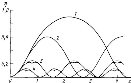
FIG. 1. Comparison of results obtained from (2.3) with the exact solution;  $\Delta s = 0.2, 1.0, 3.0,$  and  $5.0$  for curves 1, 2, 3, and 4, respectively. Broken curves show regions where the SIA differs from the exact solution.
