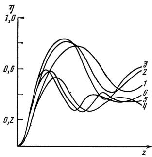
FIG. 2. Conversion coefficient  $\eta$  as a function of  $l = z/l_{ni}$  for beams modulated in space and time;  $l = 0.113$  for curves 1–3 and  $l = 0.513$  for curves 4–6.
