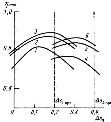
FIG. 4. Maximum conversion coefficient as a function of  $\Delta s_0$ : 1, 4—Gaussian beams; 2, 5—hypergaussian beams ( $N_1 = 4, N_2 = 2$ ); 3, 6—hypergaussian beams ( $N_1 = 6, N_2 = 2$ );  $\Delta s_{1, \text{opt}}, \Delta s_{2, \text{opt}}$ —optimum values of  $\Delta s_0$  for unmodulated waves.
