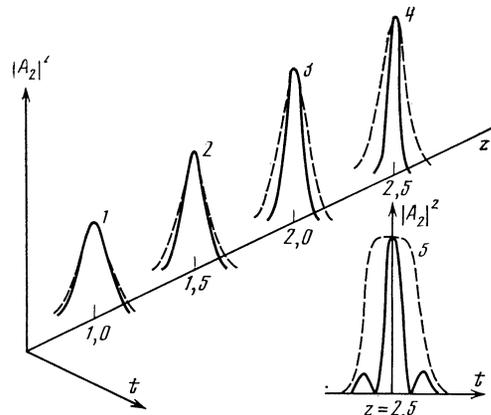
FIG. 3. Evolution of a pulse during its propagation in a nonlinear medium. Curves 1–4 correspond to the Gaussian pulse ( $N_2 = 2$ ) and curve 5 to the hypergaussian pulse ( $N_2 = 6$ ).
