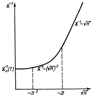
FIG. 2. The reciprocal susceptibility  $\chi^{-1}$  as function of  $H^{1/2}$ . For  $D^2 \ll H^{1/2} \ll D$  the relation  $\chi^{-1} \sim D^{-2}(H^{1/2})^3$  holds; for  $H^{1/2} \gg D$ ,  $\chi^{-1} \sim H^{1/2}$ .
