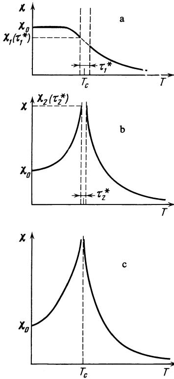
FIG. 1. Qualitative behavior of the susceptibility of a magnet (a) with random fields ( $n = 1$ )  $\chi_0 \sim D^{-4}$ ,  $\chi(\tau_1^*) \sim D^{-2}$ ,  $\tau_1^* \sim D^{3/2}$ ; (b) with a random second order anisotropy axis:  $\chi_0 \sim D^{-4}$ ,  $\chi(\tau_2^*) \sim D^{-8}$ ,  $\tau_2^* \sim D^{6/4}$ ; (c) with a random third order anisotropy axis.
