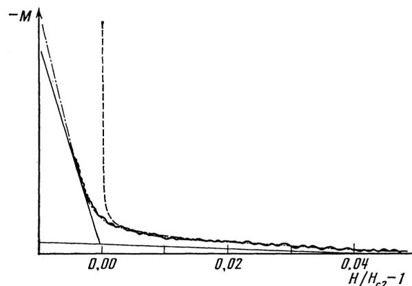
FIG. 2. Dependence of the magnetization on the magnetic field (Nb:5.7% Mo,  $T = 4.2 \text{ K}$ ): dashed curve—linear approximation, dash-dot—Hartree-Fock approximation with screened potential, solid—self-consistent-field approximation, wavy—experimental dependence.
