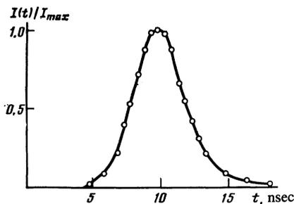
FIG. 4. The time dependence of the radiation intensity at the end of the sample: points—experiment;<sup>12</sup> curve—radiation intensity according to Eq. (3.8). Here  $\tau_D \approx 7$  ns,  $\tau_{SF} \approx 0.8$  ns,  $\tau_0 \approx 3$  ns [the parameter  $\tau_0 \approx \pm (2$  to  $3)$  ns is introduced to take into account possible systematic errors].
