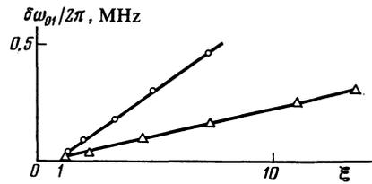
FIG. 5. Dependence of the spectral emission width  $\delta\omega_{0.1}$ , measured at the 0.1 intensity level, on the pump level  $\xi$  at  $H = 380$  Oe;  $\Delta$ — $T = 1.2$  K,  $O$ — $4.2$  K.
