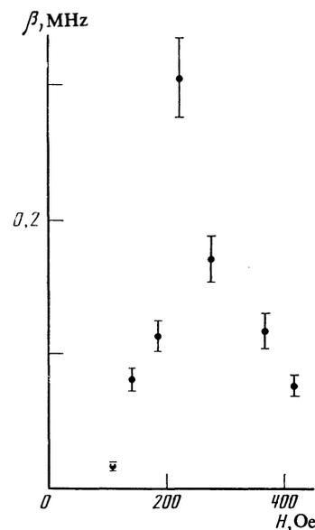
FIG. 6. Dependence of proportionality coefficient  $\beta = \delta\omega_{0.1}/(\xi - 1)$  on the magnetic field  $H$  at  $T = 1.2$  K.
