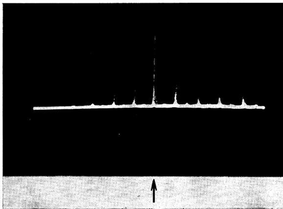
FIG. 7. Emission spectrum for  $H$  parallel to the binary axis;  $\xi \sim 2.5$ ;  $T = 1.2$  K;  $H = 300$  Oe; the arrow marks the frequency  $\omega_p/2$ .
