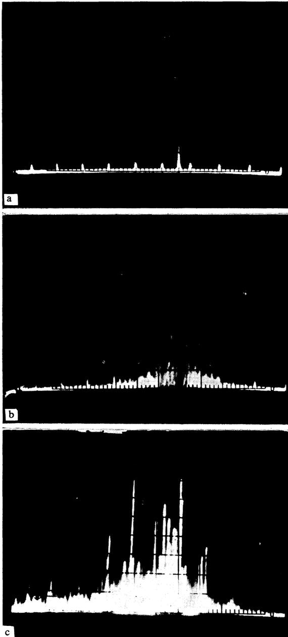
FIG. 4. Change of emission spectrum with increase of the pump level  $\xi$ : a— $\xi \sim 1.5$ , b— $\sim 5$ , c— $\sim 15$ ;  $H$  perpendicular to the binary axis,  $T = 1.2$  K,  $H = 300$  Oe. The spikes in Figs. a and b mark 1 MHz frequency intervals.
