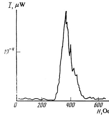
FIG. 3. Dependence of the average radiation intensity  $I$  at the receiver input on the magnetic field  $H$ ;  $\xi^2 \sim 10$ ,  $T = 1.2$  K.
