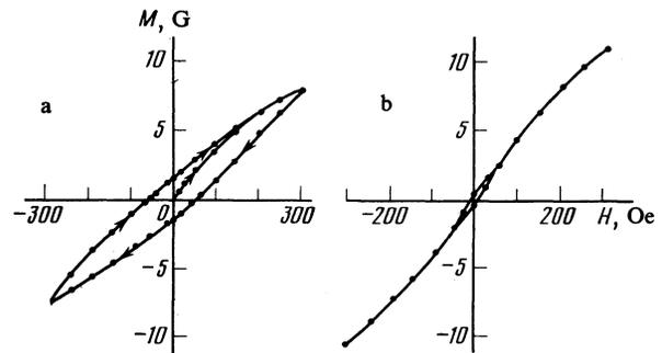
FIG. 4. Hysteresis loops of  $\text{Fe}_{65}\text{Ni}_{20}\text{Cr}_{15}$  alloys at 4.2 (a) and 15 K (b).
