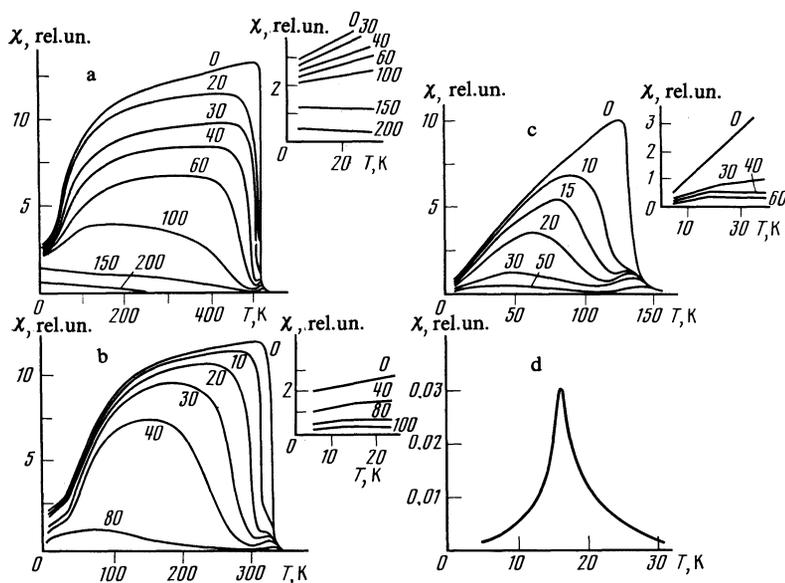
FIG. 1. Temperature dependences of the differential magnetic susceptibility of  $\text{Fe}_{65}\text{Ni}_{35-x}\text{Cr}_x$  alloys with  $x = 0$  (a), 5 (b), 10 (c) and 15 (d). The numbers on the curves indicate the value of the external constant field in Oe.
