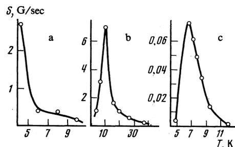
FIG. 2. Temperature dependences of the coefficient  $S$  from expression (1) for alloys with  $x = 5$  (a), 10 (b), and 15 (c).
