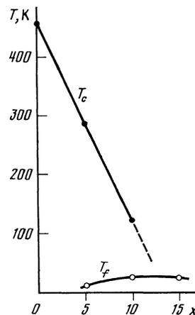
FIG. 5. Magnetic phase diagram of the system  $\text{Fe}_{65}\text{Ni}_{35-x}\text{Cr}_x$ .
