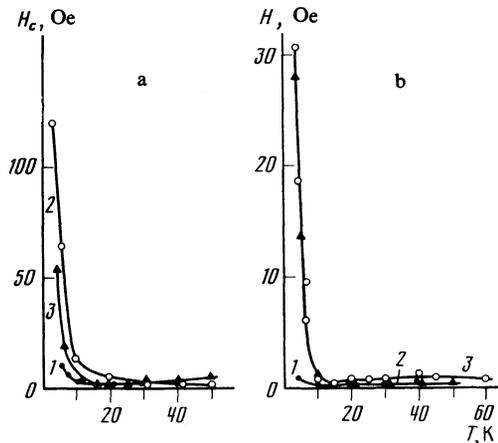
FIG. 3. Temperature dependences of the coercive force  $H_c$  (a) and of the shift  $\Delta H$  of the hysteresis curve (b) of  $\text{Fe}_{65}\text{Ni}_{35-x}\text{Cr}_x$  alloys with  $x = 5$  (1), 10 (2) and 15 (3). The shift of the hysteresis loop was measured after cooling in a magnetic field  $H_0 = 50$  (curves 1 and 2) and 20 Oe (curve 3).
