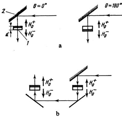
FIG. 8. Diagram of setup for the observation of resonant absorption a) for samples rotated  $180^\circ$  relative to the  $H_0^+$  direction, b) for  $180^\circ$  change of the direction of the microwave propagation.
