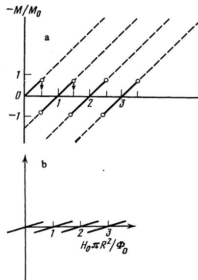
FIG. 1. Dependence of the magnetic moment of a thin superconducting cylinder on an external magnetic field  $H_0$  parallel to the cylinder axis: a) the parameter  $\mu \gg 1$ , b)  $\mu \ll 1$ .
