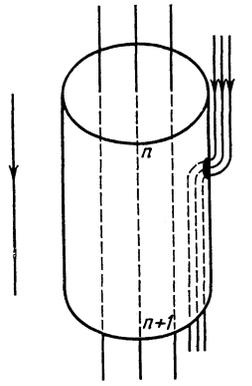
FIG. 2. Transition from a state with the number  $n$  (in the upper part of the cylinder). The normal "core" of the vortex (small black circle) moves along the cylinder whose radius is much larger than  $\delta$ .
