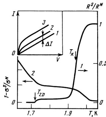
FIG. 1.—Copies of the recorded film resistance as a function of temperature. 2—Normalized conductivity of the Al-Al<sub>2</sub>O<sub>3</sub>-Bi tunnel junction in the region in which the aluminum electrode goes over into the superconducting state. The inset shows current-voltage characteristic of the aluminum film with excess current  $\Delta I$ : curve 1)  $T = 4.2 \text{ K}$ , 2)  $1.85$ , 3)  $1.74$ .
