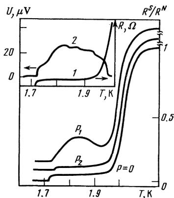
FIG. 3. Effect of 10-GHz microwave power on  $R(T)$  of the aluminum film.  $P_1 = -8$  dB,  $P_2 = -13$  dB (the superconductivity curves are shifted along the ordinate axis). The inset shows the voltage across the specimen, induced by the microwave radiation, as a function of temperature.
