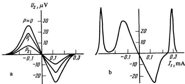
FIG. 4. a) Amplitude of the signal from the flux transformer,  $U_2(I_1)$ , as a function of the microwave power, b) anomalous behavior of the characteristic of the flux transformer.
