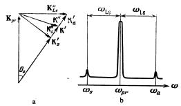
FIG. 1. a) Arrangement of wave vectors of the probing  $(\mathbf{k}_{pr})$  and scattered  $(\mathbf{k}'_{s,a})$  emissions, as well as of the plasma oscillations  $(\mathbf{k}''_{s,a})$ ; b) shape of scattering spectrum of probing emission in a homogeneous plasma in the case  $\alpha + (k'' r_{pe})^{-1} 1$ .
