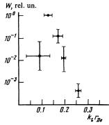
FIG. 5. Example of more complete reconstruction of the plasma-turbulence spectrum in the  $n_c/4$  region when the scattering of the probing wave is recorded in two observation directions for one of the polystyrene targets.
