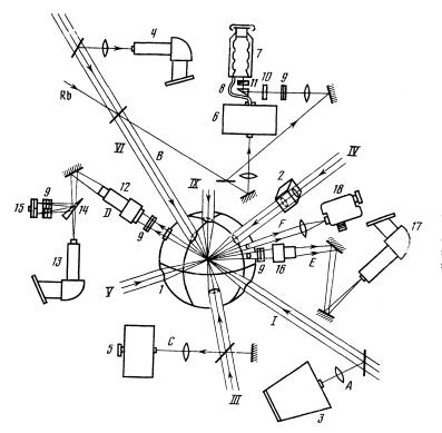
FIG. 2. Arrangement of the heating beam and of the diagnostic apparatus for the investigation of the emission of the harmonics and of the Raman scattering of the probing emission. A, B, C, D, E, F—recording channels; 1—vacuum chamber; 2—KDP crystal; 3–6, 14, 17, 18—spectrographs; 7, 8—photoelectronic recorder with light pipe; 9—light filters; 10—scatterer; 11—stepped attenuator; 12, 16—lenses; 14—optical wedge; 15—ccassette. The Roman numbers label the heating beams.
