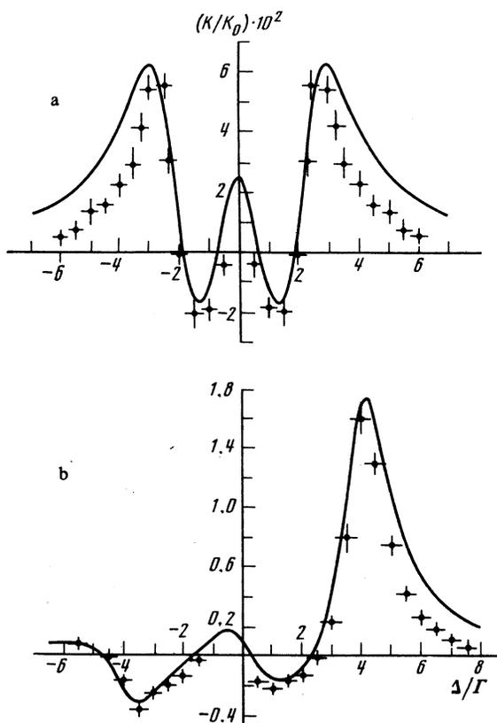
FIG. 6. Spectra of nonlinear interference effects: curves—theory, points—experiment ( $\Delta = \Omega - \omega_{21}$ ): a—resonant two-photon action of saturating noise field,  $\Delta_n = 3$  kHz,  $V^2 = 5.25 \Gamma^2$ —saturation parameter,  $\Gamma$ —natural line width,  $\varepsilon_0 = \omega_{21} - \omega_1 - \omega_0 = 0$ ; b—nonresonant action of noise field,  $n = 3$  kHz,  $V^2 = 14 \Gamma^2$ ,  $\varepsilon_0 = 1.4 \Gamma$ .
