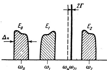
FIG. 1. Scheme for obtaining frequency-phase correlation of noise fields.  $\Delta_n$  is the spectral width of the noise radiation.
