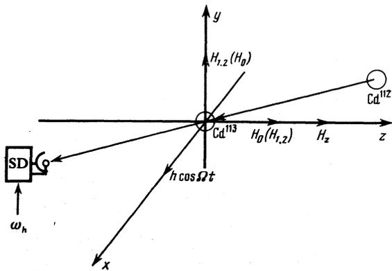
FIG. 2. Optical orientations of the  $\text{Cd}^{113}$  atoms. SD—synchronous detector.
