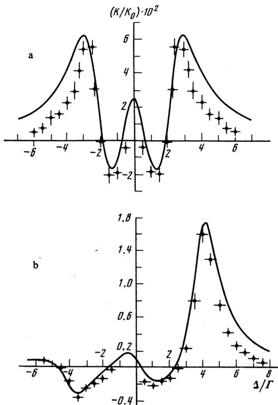
FIG. 6. Spectra of nonlinear interference effects: curves—theory, points—experiment ( $\Delta = \Omega - \omega_{21}$ ): a—resonant two-photon action of saturating noise field,  $\Delta_n = 3$  kHz,  $V^2 = 5.25 \Gamma^2$ —saturation parameter,  $\Gamma$ —natural line width,  $\varepsilon_0 = \omega_{21} - \omega_1 - \omega_0 = 0$ ; b—nonresonant action of noise field,  $n = 3$  kHz,  $V^2 = 14 \Gamma^2$ ,  $\varepsilon_0 = 1.4 \Gamma$ .
