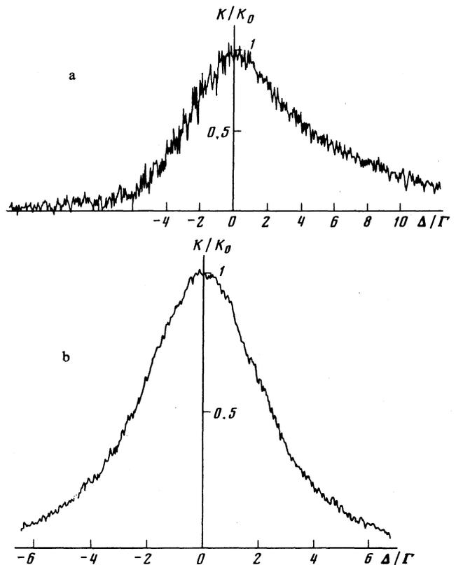
FIG. 4. Two-photon-absorption spectra of a correlated noise field: a— $\Delta_n = 300$  Hz; b— $\Delta_n = 3$  kHz.  $K$ —absorption coefficient of noise field,  $K_0$ —absorption coefficient of monochromatic field having the same intensity at the line center.  $\Delta$ —frequency detuning of the field whose absorption is investigated from the transition frequency  $\omega_{21}$ . Here  $\Delta = \omega_0 + \omega_1 - \omega_{21}$ .
