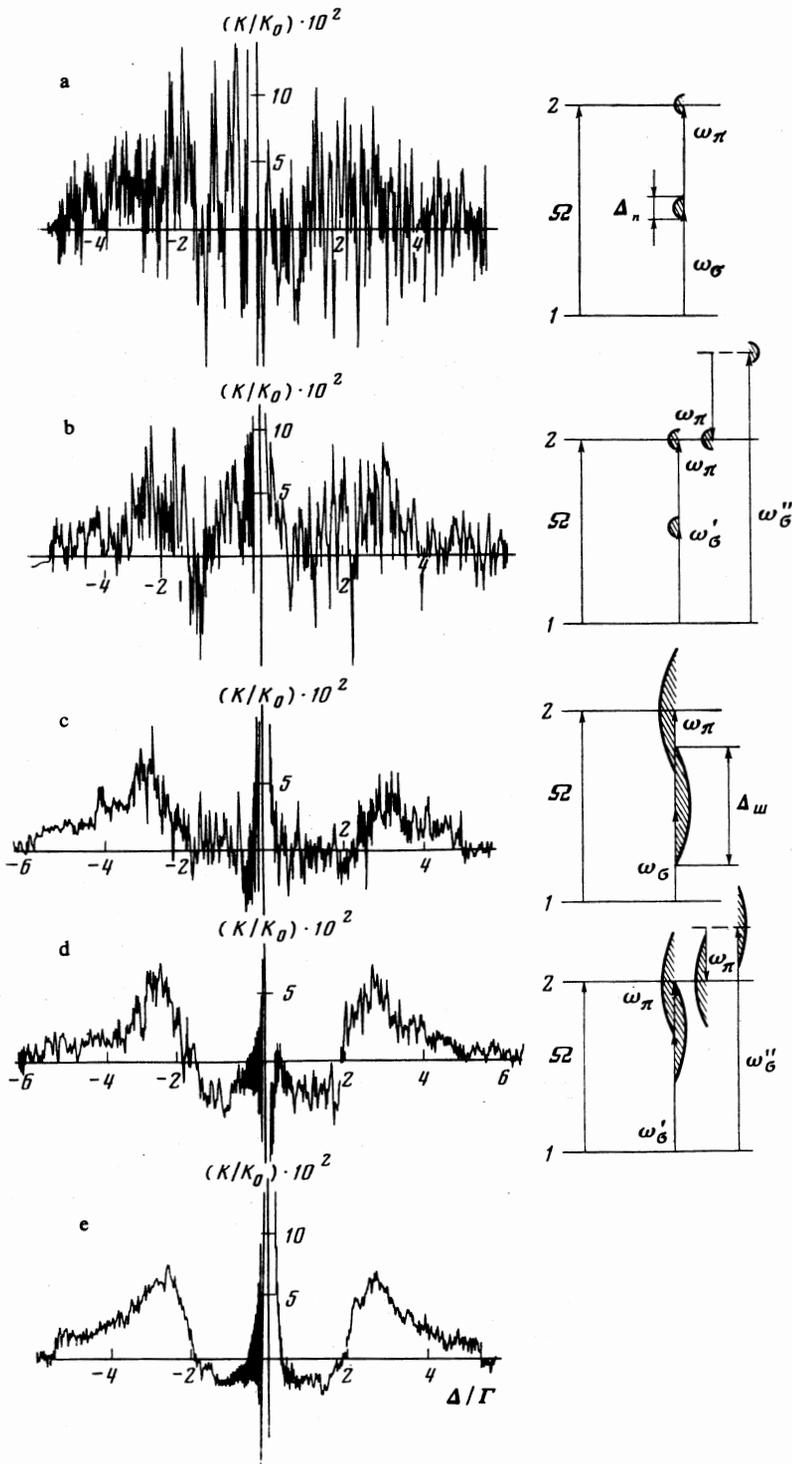
FIG. 5. Absorption spectra of weak sounding monochromatic radiation (nonlinear interference effect) for different widths of the noise-pump spectrum and different two-photon excitation mechanisms: a, b ( $\Delta_n = 300$  Hz) and c, d ( $\Delta_n = 3$  kHz)—noise pumping, e—monochromatic pumping. The shaded sections show the width  $\Delta_n$  of the noise-field spectrum;  $\Delta = \Omega - \omega_{21}$ .
