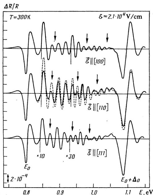
FIG. 1. ER spectra for three electric field directions. The solid line for  $\mathcal{E} \parallel [110]$  shows the spectrum recorded with a light-wave polarization vector  $e \parallel [001]$ , and the dashed—with  $e \parallel [110]$ . The two other spectra are independent of polarization. The arrows mark the positions of the "beats."
