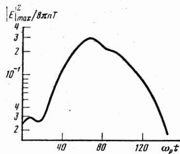
FIG. 3. Energy density of the oscillations at the center of the cavity as a function of the time.
