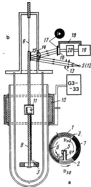
FIG. 1. a) Arrangement of ring; b) arrangement of apparatus and of the automatic recording of oscillations of the system.
