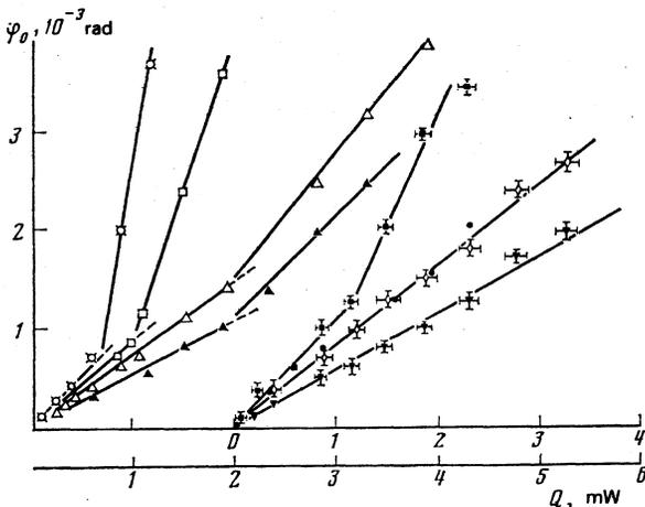
FIG. 2. Dependence of amplitude of oscillations  $\varphi_0$  on the power  $Q$  dissipated in the heater, for various bath temperatures:  $\circ$ —1.40 K,  $\times$ —1.46 K,  $\square$ —1.55 K,  $\blacksquare$ —1.74 K,  $\blacktriangle$ —1.90 K,  $\triangle$ —1.96 K,  $\bullet$ —2.06 K,  $\diamond$ —2.10 K,  $\blacktriangledown$ —2.15 K.
