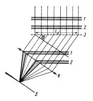
FIG. 6. The scheme of performance of spectral apparatus: 1, 2 section of reflected radiation with equal instant frequency, 3— diffraction grating, 4—lens, 5—screen.
