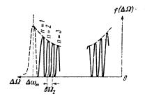
FIG. 5. The spectral density of the square of the electric field intensity of the reflected wave  $f(\Delta \Omega)$ .
