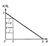
FIG. 1. Plasma concentration  $N/N_c$  vs coordinate for the instants of time t = 0 and  $t \rightarrow \infty$ .
