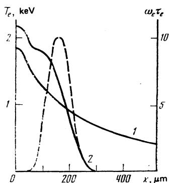
FIG. 5. Transverse profiles of  $T_e$  and  $|\omega_e \tau_e|$  at  $b = 33 \mu\text{m}$ ,  $q_0 = 4.5 \times 10^{14} \text{ W/cm}^2$ , and  $t = 0.3 \text{ nsec}$  near the critical surface. The dashed line is the profile of  $|\omega_e \tau_e|$ . Curves 1 and 2 correspond to calculations without and with generation of magnetic fields.
