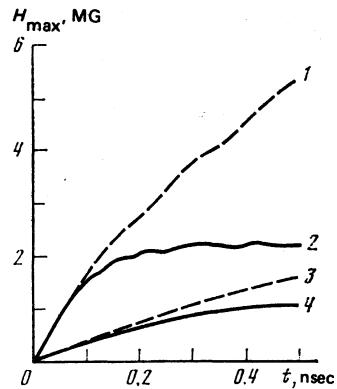
FIG. 1. Time dependence of the maximum value of the magnetic field. The dashed and solid lines correspond respectively to the magnetothermal and complete formulations. Curves 1 and 2 correspond to  $b = 33 \mu\text{m}$  and  $q_0 = 4.5 \times 10^{14} \text{ W/cm}^2$ , and curves 3 and 4 to  $b = 200 \mu\text{m}$  and  $q_0 = 0.75 \times 10^{14} \text{ W/cm}^2$ .
