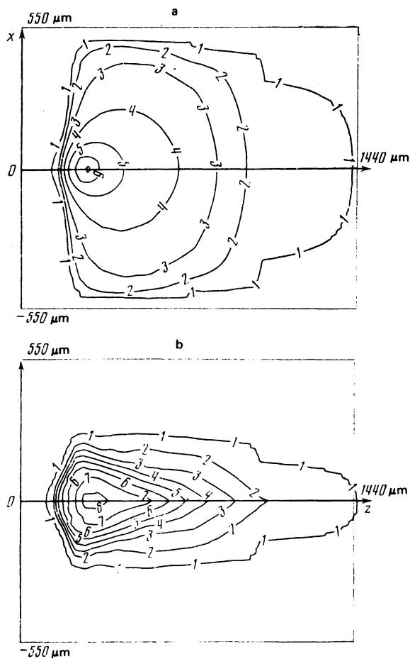
FIG. 4. Level lines of electron temperature at  $b = 33 \mu\text{m}$ ,  $q_0 = 4.5 \times 10^{14} \text{ W/cm}^2$ , and  $t = 0.3 \text{ nsec}$ . The case *a* pertains to the calculation without allowance for the generation and magnetic field, and case *b* to the complete formulation. The curve with index 1 corresponds to  $T_e = 0.025$ , 2—0.3, 3—0.6, 4—0.9, 5—1.2, 6—1.5, 7—1.8, and 8—2.1 keV.
