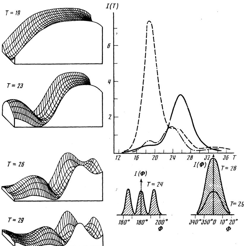
FIG. 3. Relaxation of sample measuring  $25 \times 1.75 \lambda^2$ . On the right is shown the temporal variation of the intensity of the radiation in different directions and the angular structure of the radiation at various instants of time; solid curve— $\Phi = 0^\circ$ , dashed— $\Phi = 180^\circ$ , dash-dot— $\Phi = 180^\circ \pm 14^\circ$ .
