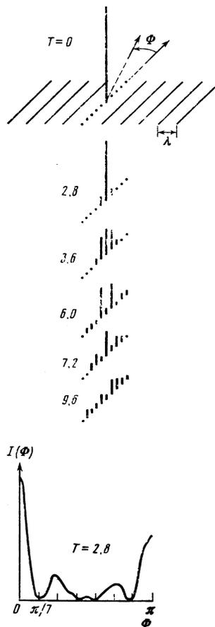
FIG. 5. Spontaneous decay of one excited radiator in the same lattice ( $\lambda, \lambda/4$ ) as in Fig. 4. The dynamics of the excitation of the radiators in the Bragg plane containing the excited radiator is shown. Below is represented the angular distribution of the intensity of the radiation. The remaining radiators located in other planes are much less excited, but their fields are in phase, and this is in fact the cause of the "screening" of the radiation.
