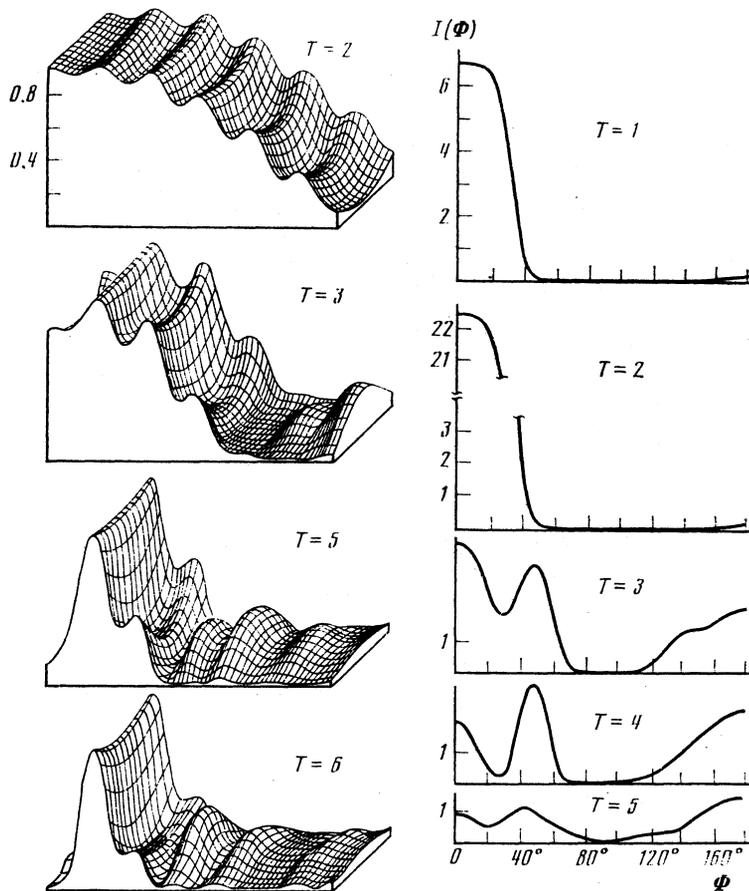
FIG. 1. Relaxation of an active sample with dimension  $3 \times 0.6 \lambda^2$ , excited by a resonant pump pulse directed along the sample. On the left is shown the temporal dynamics of the inverted population, and on the right the angular distribution of the intensity of the radiation at various instants of time. The angle  $\Phi$  is measured from the longitudinal axis of the sample, along which the exciting pulse is directed;  $T = t(\pi d^2 k^2 \rho L b / 10 \hbar)$ .
