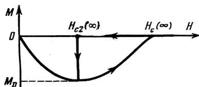
FIG. 4. Typical field dependence of the diamagnetic moment  $M$  as experimentally observed in tin.<sup>1</sup>
