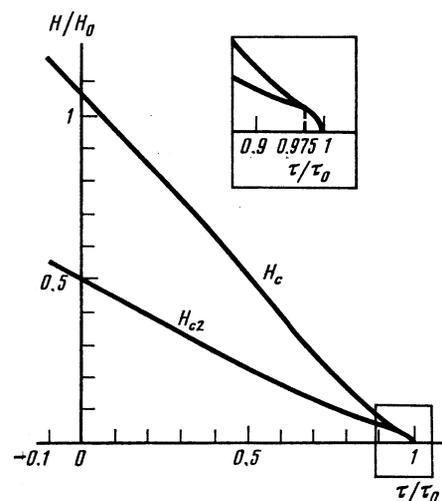
FIG. 2. Phase diagram of the localized superconductivity of the TP in tin for a parallel magnetic field (the field is in units of  $H_0 = \Phi_0 \tau_0 / \xi_0^2$ ).  $H_c$  is the critical field for the first-order transition and  $H_{c2}$  is the supercooling field. The inset shows the region around the tricritical point.
