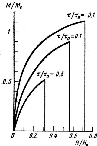
FIG. 3. Dependence of the diamagnetic moment  $M = HL(H)$ , in units of  $M_c = (2\tau_0\pi N/m)^{1/2}$ ,  $H_c = 2\tau_0(\pi N/\eta)^{1/2}$ , on the magnetic field at different temperatures for the infinite twinning plane.
