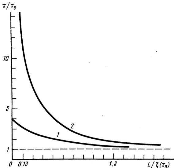
FIG. 1. Dependence of the critical temperature for the onset of LS on the distance  $L$  between two parallel TP (curve 1) and on the period  $L$  of an infinite series of TP, as well as on the thickness  $L$  of a film containing one TP (curve 2).
