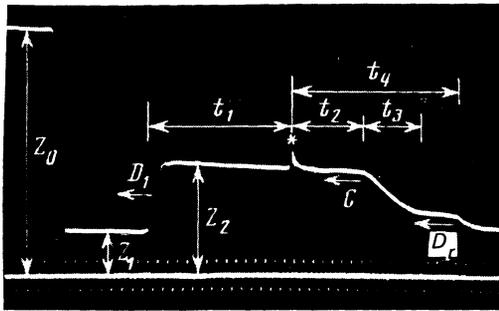
FIG. 3. Profiles of compression and rarefaction waves in bismuth.  $D_1$ —compression shock wave of amplitude 9.28 GPa,  $C$  and  $D_r$ —elastic-plastic and rarefaction shock waves.
