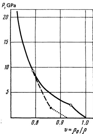
FIG. 6.  $P(v)$  plot of bismuth: solid curve—experimental shock adiabat of bismuth from Ref. 15, dashed curve—calculated expansion isentrope, dotted curve—rarefaction shock wave ( $D_r = 1.6$  km/sec).
