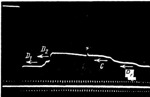
FIG. 4. Profiles of compression and rarefaction waves in bismuth:  $D_1$ —compression shock wave of amplitude 2.5 GPa,  $D_2$ —second compression shock wave of amplitude 5.8 GPa,  $C$  and  $D_r$ —rarefaction elastoplastic and shock waves.
