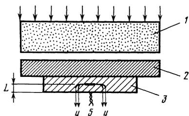
FIG. 1. Experimental setup to reveal the two-wave configuration of the compression shock front and the rarefaction wave profile in bismuth: 1—explosive charge of 90 mm diameter, 2—metallic screen 10 mm thick, 3—bismuth sample, 4—manganin pressure sensor, 5—electric contact-making sensor.
