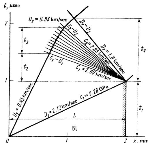
FIG. 5.  $x-t$  diagram of the processes of shock compression and subsequent relaxation of bismuth.
