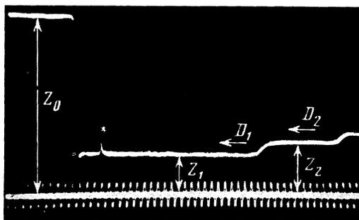
FIG. 2. Two-wave configuration of shock front in bismuth. Amplitude of first compression wave  $2.55 \pm 0.05$  GPa, of second wave  $4.4 \pm 0.1$  GPa.
