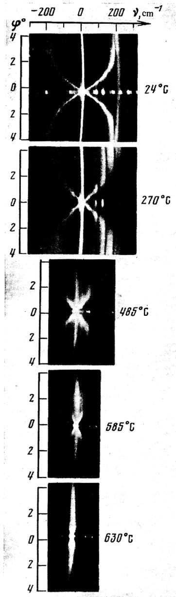
FIG. 2. Frequency-angle spectra of RS of light by polaritons of the lower branch, which are coupled with the soft mode of symmetry  $A_1(z)$  of the lithium-tantalate crystal.  $\nu$  is the frequency shift of RS and  $\varphi$  is the scattering angle reckoned inside the crystal. The spectra were obtained at crystal temperatures  $24, 270, 485, 585,$  and  $630^\circ\text{C}$ .
