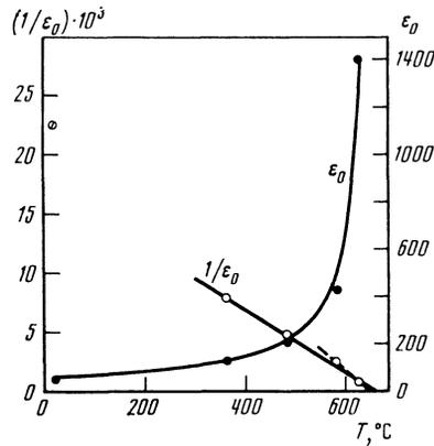
FIG. 3. Temperature dependence of static dielectric constant  $\epsilon_0(T)$ . Points—measurement results. Solid curve—calculation using linear approximation of the temperature dependence of the reciprocal of the dielectric constant  $1/\epsilon_0$ , obtained using four experimental points. The dashed straight line is drawn through the two points obtained at the highest temperatures of the crystal.
