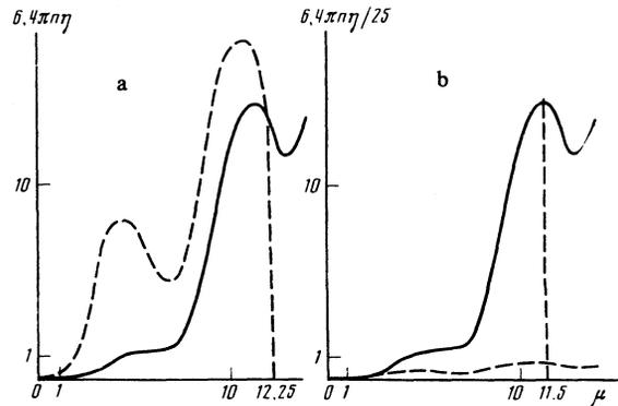
FIG. 2. Efficiency  $\eta$  as a function of the saturation parameter  $\mu$  in FEL with “short” (dashed curves) and “long” (solid curves) undulators at different (a) and identical (b) gain levels in a weak field.
