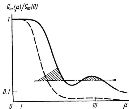
FIG. 3. Gain, normalized to unity as  $\mu \rightarrow 0$ , in an FEL with a “short” (dashed curves) and a “long” (solid) undulators.
