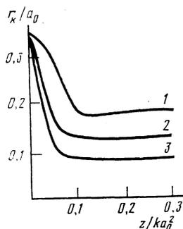
FIG. 3. Correlation range in the propagation direction near the beam axis vs  $z/ka_0^2$  for  $N = 3$ ,  $\delta = 0$ , and the following values of  $p$ : 1-10, 2-20, 3-40.
