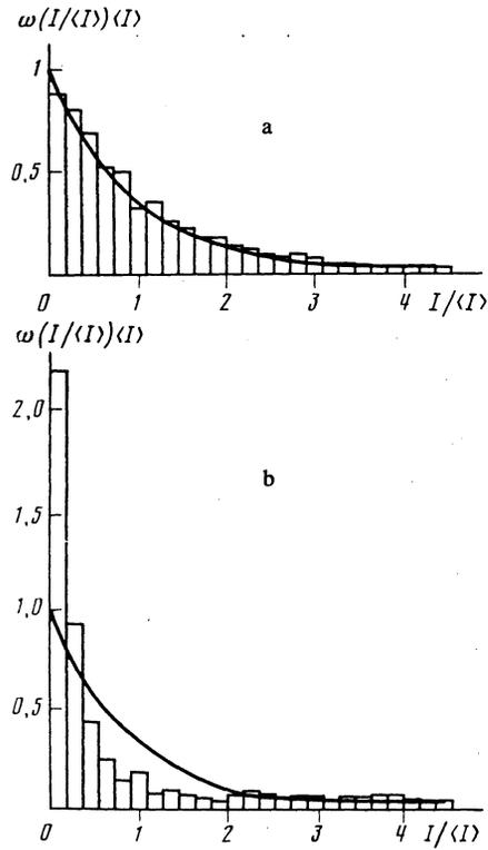
FIG. 1. Probability density distribution for the intensity on the axis of a narrow-band beam ( $\delta = 0$ ) for  $p = 40$  and  $N = 3$  at the points  $z = 0$  (a) and  $z = 0.15ka_0^2$  (b).
