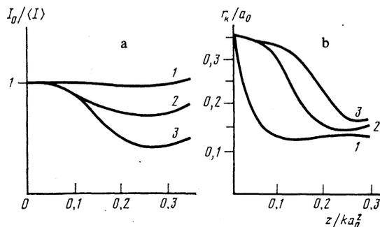
FIG. 4. Intensity (a) and correlation range (b) on the beam axis vs  $z/ka_0^2$  for  $N = 3$ ,  $p = 20$ , and the following values for the width  $\delta$  of the frequency spectrum: 1-0, 2-10, 3-100.
