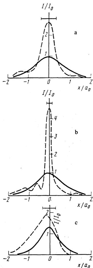
FIG. 2. Average (solid curves) and instantaneous (dashed curves) intensity profiles for a beam with  $p = 20$  and  $N = 3$  at the entrance to the medium (a) and at the point  $z + 0.15ka_0^2$  for  $\delta = 0$  (b) and  $\delta = 100$  (c).
