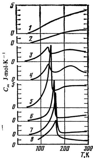
FIG. 2. Magnetic component of the heat capacity of  $(\text{Pd}_x\text{Pt}_{1-x})_3\text{Fe}$  alloys vs temperature. Curve 1 corresponds to  $x = 0.62$ ; 2—0.57; 3—0.53; 4—0.49; 5—0.47; 6—0.31; 7—0.16; 8—0.
