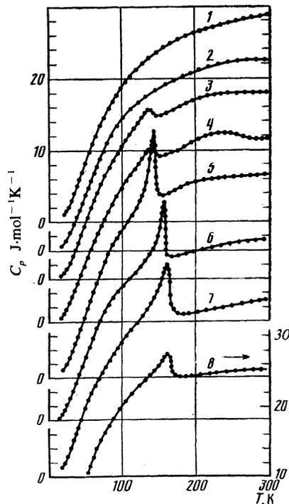
FIG. 1. Heat capacity of the alloys  $(\text{Pd}_x\text{Pt}_{1-x})_3\text{Fe}$  vs temperature. Curve 1 corresponds to  $x = 0.62$ ; 2—0.57; 3—0.53; 4—0.49; 5—0.47; 6—0.31; 7—0.16; 8—0.
