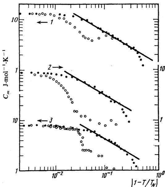
FIG. 4. Magnetic component of the heat capacity of the alloys  $(\text{Pd}_x \text{Pt}_{1-x})_3\text{Fe}$  vs  $|1 - T/T_N|$ . The dark and light circles are for  $T < T_N$  and  $T > T_N$ , respectively. The values 1, 2, 3, correspond to  $x = 0.16, 0.31$ , and  $0.47$ , respectively. The solid line is a plot of (1) at  $\alpha = 0.58$ .
