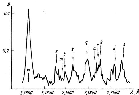
FIG. 3. Density pattern of the Cr-XXIII spectrum, obtained after nine discharges with additional electron-cyclotron heating of  $500 \text{ kW}$  power. Plasma parameters:  $T_e = 2.4 \text{ keV}$ ;  $n_e = 3 \times 10^{13} \text{ cm}^{-3}$ .
