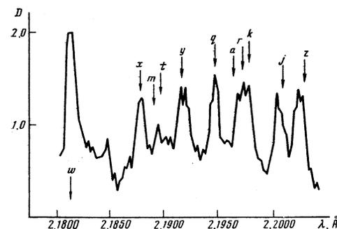
FIG. 4. Density pattern of Cr-XXIII spectrum obtained after nine discharges with different plasma-heating conditions.
