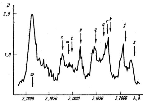
FIG. 2. Density pattern of Cr-XXIII spectrum obtained after eight discharges with ohmic heating by a current  $\sim 250 \text{ kA}$ . Plasma parameters:  $T_e = 1.5 \text{ keV}$ ;  $n_e = 2 \times 10^{13} \text{ cm}^{-3}$ .
