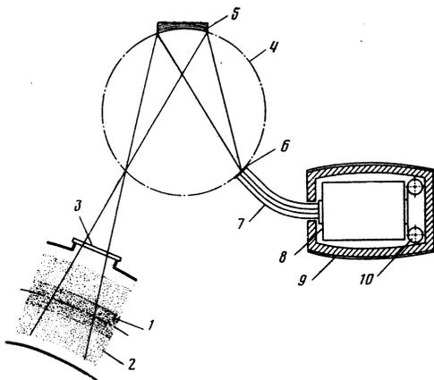
FIG. 1. Setup for the registration of the x rays: 1) hot plasma; 2) peripheral zone; 3) beryllium window; 4) Rowland circle; 5) dispersing crystal; 6) converter screen; 7) fiber optics; 8) light intensifier; 9) multilayer magnetic shield; 10) photographic film.
