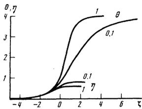
FIG. 3. Structure of ionization-wave front. Dependence of the dimensionless radiation of the plasma temperature from its maximum value  $\theta$  and of the dimensionless intensity of the electromagnetic radiation  $\eta$  on the dimensionless coordinate  $\zeta$  at two values of the parameter  $b \equiv \kappa_0/\kappa_m$  ( $b=1$  and  $0.1$ ).  $2(k\delta_m)^2=0.89$ ;  $\omega=\nu$ ;  $I/T_m=8$ ;  $T_0/T_m=4 \times 10^{-3}$ .
