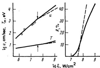
FIG. 4. Dependence of the ionization-wave velocity, plasma temperature behind the front, and the reflectivity of the front on the neodymium-laser radiation intensity. Glass ZhS-12. The dashed lines show the results of the calculation performed in the geometric-optical approximation. The solid lines are the results of the solution of the complete system of Maxwell's equations. The points are experimental.<sup>7,8</sup>
