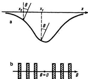
FIG. 3. Wavefront profile (a) and interference pattern in the far zone (b) for the one-dimensional problem.
