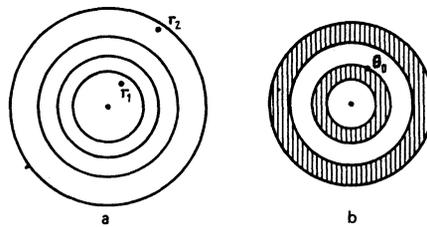
FIG. 4. Constant-depth lines of the wave-front surface (a) and interference pattern in the far zone (b) in the axially symmetrical problem.
