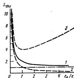
FIG. 1. Dependence of the threshold power  $S_{\text{thr}}$  (in units as  $\varepsilon_a/\varepsilon_{\perp} \rightarrow \infty$ ) on the value of  $\varepsilon_a/\varepsilon_{\perp}$  for broad beams. Curve 1 describes the correct behavior of the threshold,<sup>9</sup> curve 2 shows the behavior of the threshold according to the equations of Refs. 11 and 13, while curve 3 shows the same for Ref. 12.
