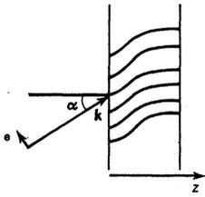
FIG. 6. NLC cell with perturbed director orientation, on which a light wave is incident from air at an angle  $\alpha$ .
