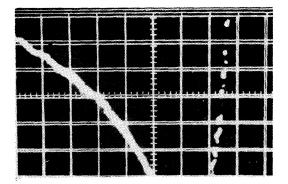
FIG. 3. Oscillogram of the signal of acoustic emission accompanying the emergence of a dislocations pile-up formed with the surface to this surface. The minimum scale division along the abscissa is  $8 \mu s$ .
