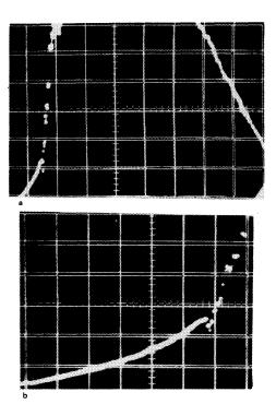
FIG. 2. Oscillogram of the signal of acoustic emission accompanying the approach of the pile up of dislocations from the interior of the crystal to the surface with its subsequent emergence to the surface: a) the minimum scale division along the abscissa in  $8 \ \mu$ s; b) the minimum scale division along the abscissa is  $1.6 \ \mu$ s.
