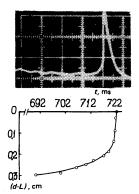
FIG. 1. Time dependence of the distance from the tip of the twin to the surface of the crystal (d-L) juxtaposed with the oscillogram of the sound emission in the same time scale. The scale of the oscillogram along the abscissa is  $5 \,\mu$  s/cm.
