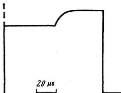
FIG. 6. Oscilloscope trace of microwave pulse traversing the resonator with the specimen for  $h > h_c^*$ .
