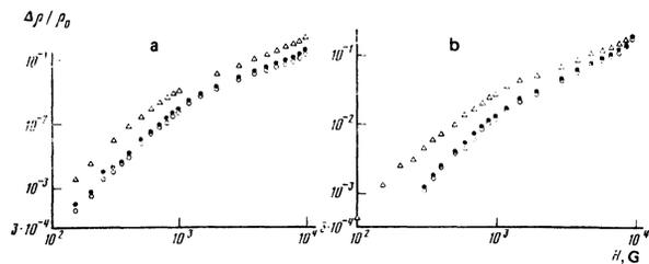
FIG. 5. Dependences of the magnetoresistance  $\Delta\rho/\rho_0$  on the magnetic field applied to control and plastically deformed samples. The deformation took place in the  $\alpha$ -bending orientation: a) at a low rate; b) at a high rate. The curves were similar for the case of  $\beta$  bending.  $\Delta$ ) Control sample;  $\circ$ ) plastically deformed longitudinal sample;  $\bullet$ ) plastically deformed transverse sample.
