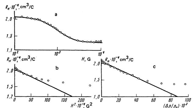
FIG. 3. Dependences of the Hall coefficient  $R_H$  for sample No. 12: a) on the magnetic field; b) on the magnetic field in the range of weak fields; c) on the magnetoresistance  $\Delta\rho/\rho_0$  in the range of weak fields.
