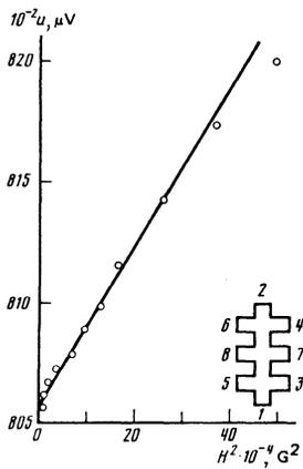
FIG. 1. Dependence of the magnetoresistance emf on the magnetic field obtained in weak fields for sample No. 12;  $H$  is the magnetic field and  $u$  is the magnetoresistance emf.
