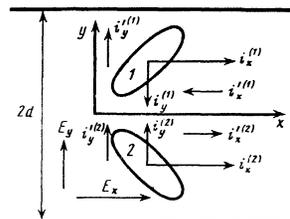
FIG. 1. Fields and partial currents in a two-valley semiconductor.
