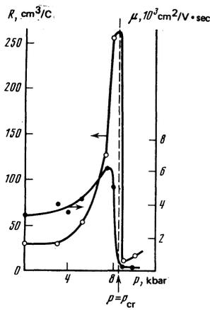
FIG. 5. Baric dependences of the Hall coefficient  $R$  and of the mobility  $\mu$  at  $T = 4.2$  for sample No. 1.
