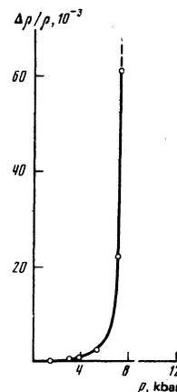
FIG. 4. Dependence of the amplitude  $A = \Delta\rho/\rho$  of the SdHO in a fixed magnetic field  $H_0 = 30 \text{ kOe}$  on the pressure  $p$  for sample No. 1.
