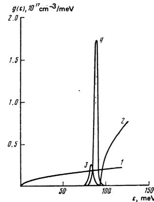
FIG. 8. State density in the impurity band of GaSb:Te: 1)  $\Gamma$  band, 2)  $L$  band (for one extremum), 3) impurity band, sample 1, 4) impurity band, sample 5.
