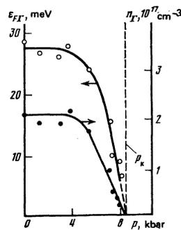
FIG. 3. Baric dependences of the density  $n_{\Gamma}$  and of the Fermi energy  $\epsilon_{F\Gamma}$  of the  $\Gamma$  electrons of sample No. 1.
