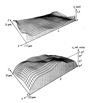
FIG. 1. Distributions of temperature and density constructed with automated processing of pin-hole-camera photographs by computer (aluminum target, E = 100 J,  $\tau = 3.0$  nsec).
