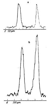
FIG. 5. Densitometer traces characterizing the distributions of intensity of the laser radiation at the focal spot (a) and sources of x radiation in the plasma corona (b) (aluminum target, E = 100 J,  $\tau = 3.0$  nsec).
