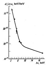
FIG. 4. Spectral distribution of intensity of x radiation of the plasma corona (aluminum target, E = 140 J,  $\tau = 3.0$  nsec).
