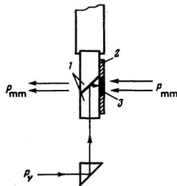
FIG. 1. Schematic drawing of the specimen holder and of the path of the beams of optical pumping and of millimeter radiation. 1) corundum prisms; 2) diaphragm; 3) specimen.
