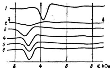
FIG. 3. Same as in Fig. 2, but for AFMR of the type  $\omega_z$ . Specimen  $2 \times 1.5 \times 0.115$  mm,  $f = 372$  GHz; lines 3-6 recorded at 2-minute intervals after turning off of the laser. The arrows indicate the instants of turning on and of turning off of the laser.
