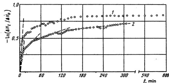
FIG. 9. Variation of  $\ln(\Delta H_t / \Delta H_0)$  with time, where  $H_0, t$  is the difference of the resonance field of the new AFMR signal at the instant of time  $t_0$  or  $t$  with respect to the original value before pumping. Signal  $\omega_{xy}$ ;  $f = 210 \text{ GHz}$ ,  $T = 5 \text{ K}$ . Pumping parameters:  $P_p = 250 \text{ kW}$ ,  $\Omega = 25 \text{ Hz}$ ,  $t_{\text{pump}} = 240 \text{ sec}$ . 1) specimen thickness  $0.11 \text{ mm}$ ; 2)  $0.92 \text{ mm}$ .
