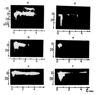
FIG. 6. Time-resolved spectrograms of scattered radiation at the fundamental frequency  $\omega_0$  (a, b, c) and at the second harmonic  $2\omega_0$  (d, e) for three angles of incidence: a) backscattering; b), d) normal to the target; c), e) specular reflection. Angle of incidence of the target 22.5°.
