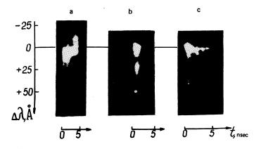
FIG. 4. Time-resolved spectrograms of radiation scattered at the fundamental frequency for normal incidence and three observation angles: a) backscattering; b)  $45^{\circ}$ ; c)  $22^{\circ}$ .
