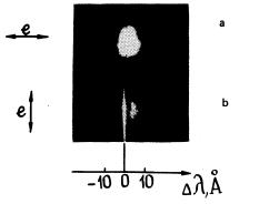
FIG. 5. Spectrograms of backscattered radiation at the fundamental frequency for two polarizations (relative to the polarization of the incident laser radiation): a) perpendicular; b) parallel.
