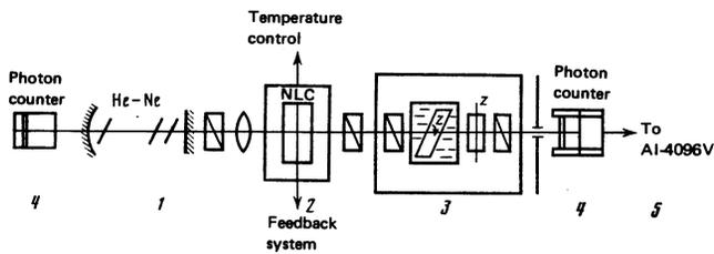
FIG. 1. Block diagram of the experimental setup.
